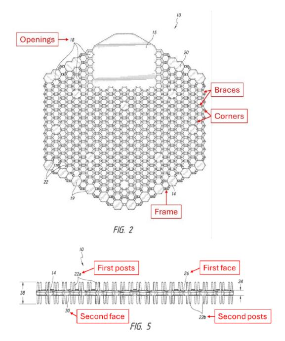
Ex. 1001, FIGS. 2 and 5.<sup>1</sup> Figure 2 provides a top view and Figure 5 provides a side view of a urinal screen according to the '098 patent. The urinal screen is described as having a frame with a first face and a second
