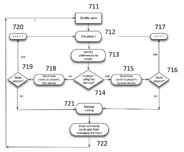
Figure 7 illustrates a flowchart showing the flow of control in an embodiment of the invention. *Id.* The illustrated flowchart 710 shows that the game server shuffles the cards (rectangle 711). *See id.* at 4:6–7. Then, for each player (ovals 712, 717, 720), the game server sequentially identifies
