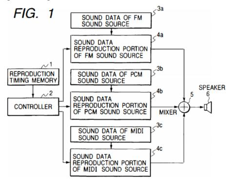
Figure 1 depicts a communication controller and ringing sound generator of a cellular phone. *Id.* at 2:59–61, 4:34–36. The ringing sound generator includes frequency modulation (FM) sound data memory 3a, pulse-code modulation (PCM) sound data memory 3b of a sound source, and Musical
