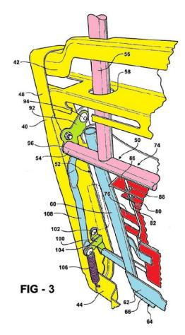
Figure 2 of the '397 patent illustrates the support frame and activation mechanism of the head restraint.
